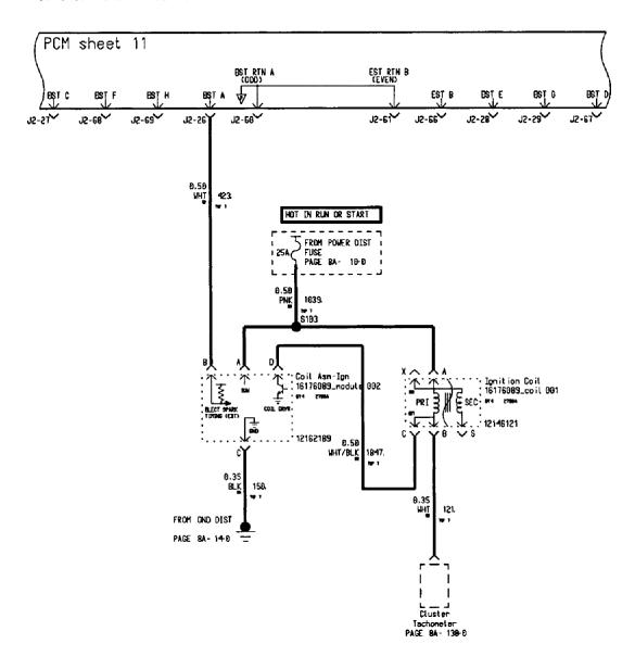
Figure 3.2.1a - XII - P/Truck - Mechanization Diagram - Engine Ignition System
